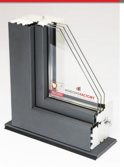
GEMINI Passiv, as a certified component of Passivhaus In stitut, meets its requirements for passive housing, that is: Uw  $0.80 \text{ W/(m}^2\text{K})$  in combination with triple-glazing Ug =  $0.7 \text{ W/m}^2\text{K}$ .
